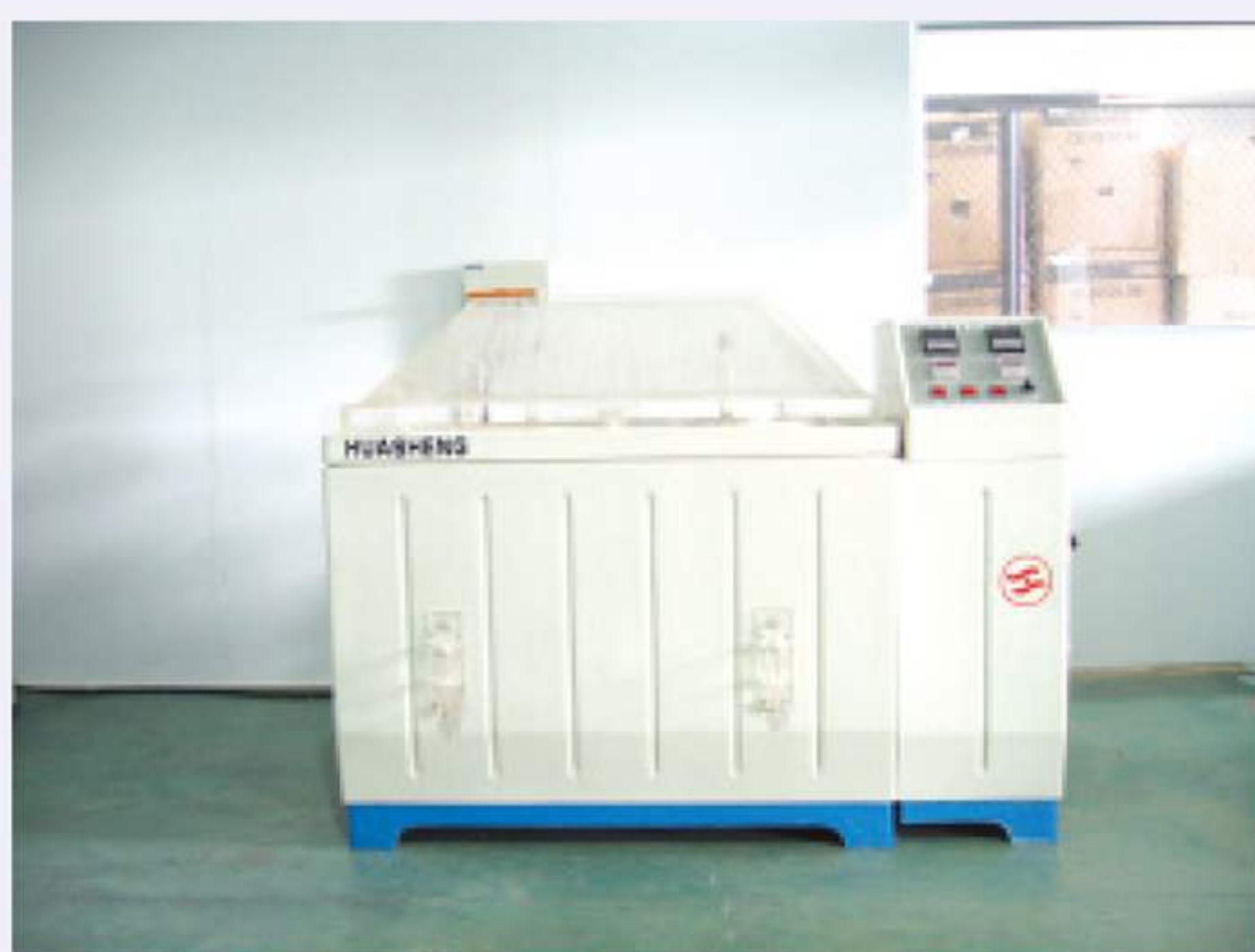
盐雾腐蚀试验箱 Corrosive salt spray chamber
